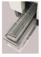
The load vessel accepts up to 60 slides and can be filled with reagent – increases throughput and allows for wet or dry coverslipping.
