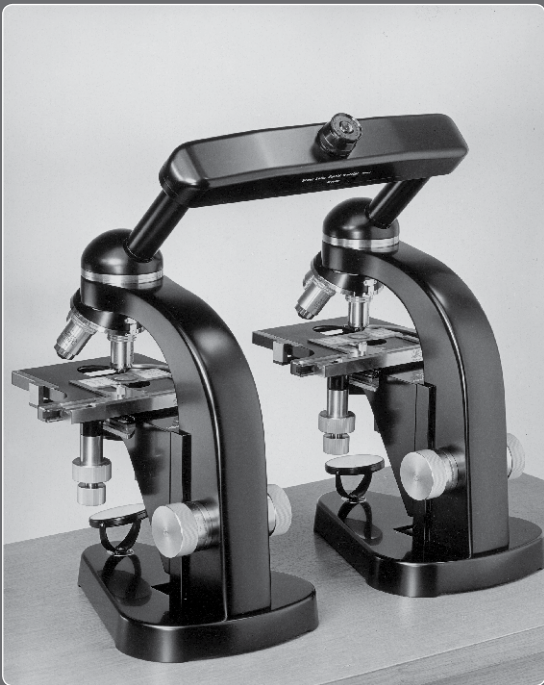
Monocular comparison microscope by Ernst Leitz, Wetzlar, year of construction 1955
