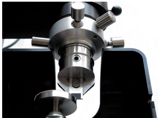
Sample holder attached on the alignment accessory. The micro-targets can be aligned during the process while observing with the stereo microscope.
